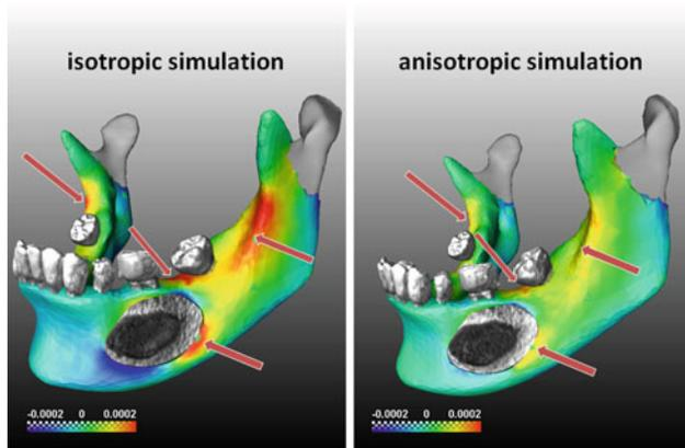
**Fig. 1** Volumetric strain based on homogeneous elastic coefficients, from simulations with isotropic (*left*) and anisotropic (*right*) material properties
